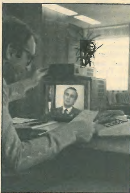
Multipurpose optical fibre networks will make 5MHz colour videophones commonplace. Prototype equipment installed over the next few years for field trials in Berlin, Düsseldorf, Hamburg, Hanover, München, Nürnberg and Stuttgart provides both telecommunication services (viewdata, speech, data, text, graphics) and broadcast services (two to four television programmes, 24 radio programmes). The DM150 million project is part of a general increase in telecom r & d spending in Germany in a drive to increase competitiveness. The networks are in addition to coaxial cable pilot projects already under way in Ludwigshafen and Dortmund, with München, Berlin and seven other cities to follow. Original area-wide plans were scrapped about two years ago and work is now limited to "islands of partial networks". With national coverage estimated to cost DM20 to 30 billion and optical systems at several times as much, the Bundespost is hoping for large price reductions with volume in the near future.
