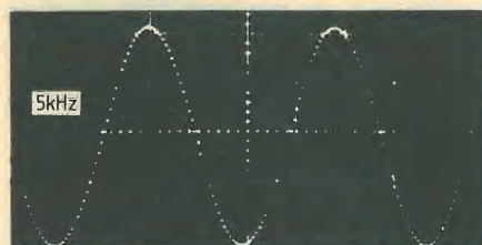
Fig.3. Oscillograms for oscillator frequencies between 5Hz and 16kHz. A single sweep time-base was used for all but the 16kHz wave-form in order to show the steps (the steps are not necessarily synchronous with the output frequency).
